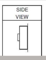
The 211SM is a surface mount, ADA compliant cabinet, measuring 11.25'' (h) x 11.25'' (w) x 3.25''(d). The unique mounting holes and free laying decal allow for a variety of door orientation options; left, right, top, or bottom.
